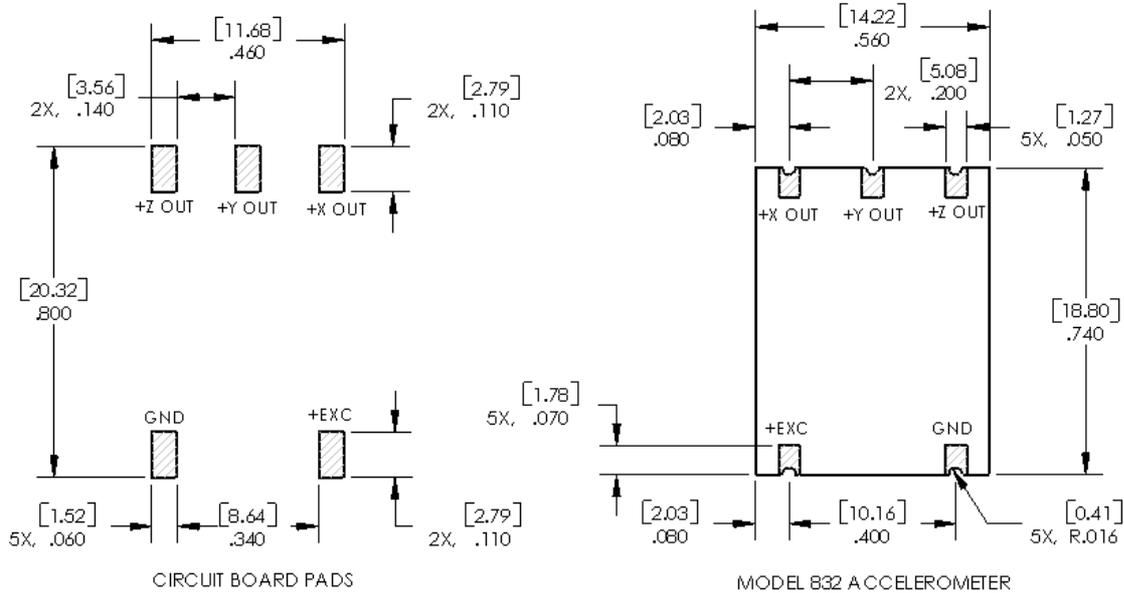
If the accelerometer is to be subjected to high amplitude shocks during operation then a thin layer of epoxy should be applied underneath the accelerometer after solder reflow attachment. A cyanoacrylate with an operating temperature up to +125°C is recommended.
