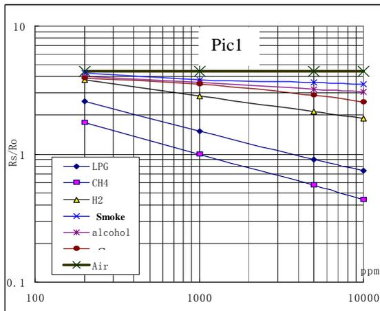
Pic1:  $R_s$  expresses the resistance of sensor in different concentration of gas.  $R_o$  expresses the resistance of sensor in 1000ppm CH<sub>4</sub>. All the tests in the picture are all finished under the standard testing condition.
