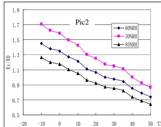
Pic2:  $R_s$  expresses the resistance under 1000ppmCH<sub>4</sub> and various temperature and humidity conditions.  $R_o$  expressed the resistance under 1000ppmCH<sub>4</sub> and 20°C/65%RH conditions.
