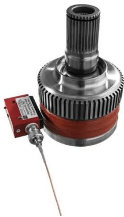
Figure 2: Compensated transmission flange with inductive supply antenna (further miniaturization of the antenna possible))
