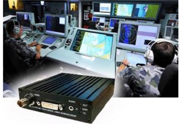
Delta Digital Video's Model 4480E H.264 HD/SD Video Encoders will be integrated into the CCTV System allowing multiple sources of combat system and other video to be converted and input into the CCTV network to be delivered into the Operations Room and throughout the ship.
