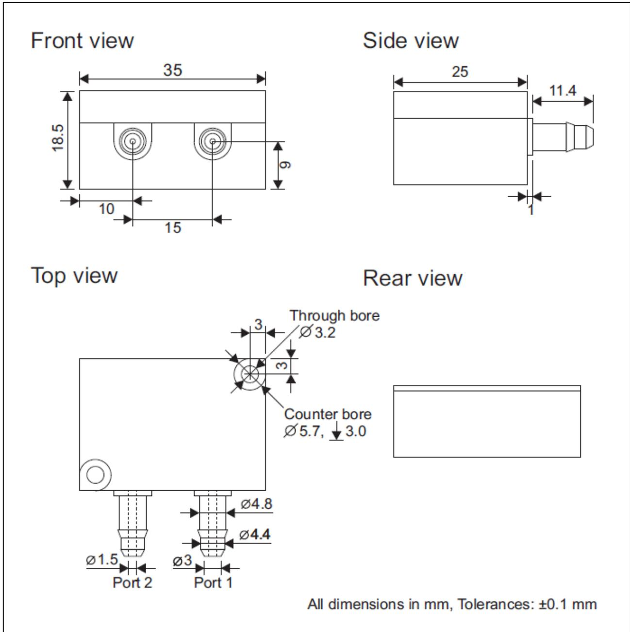
Figure 2: Dimensions and pinout of AMS 4516 package
