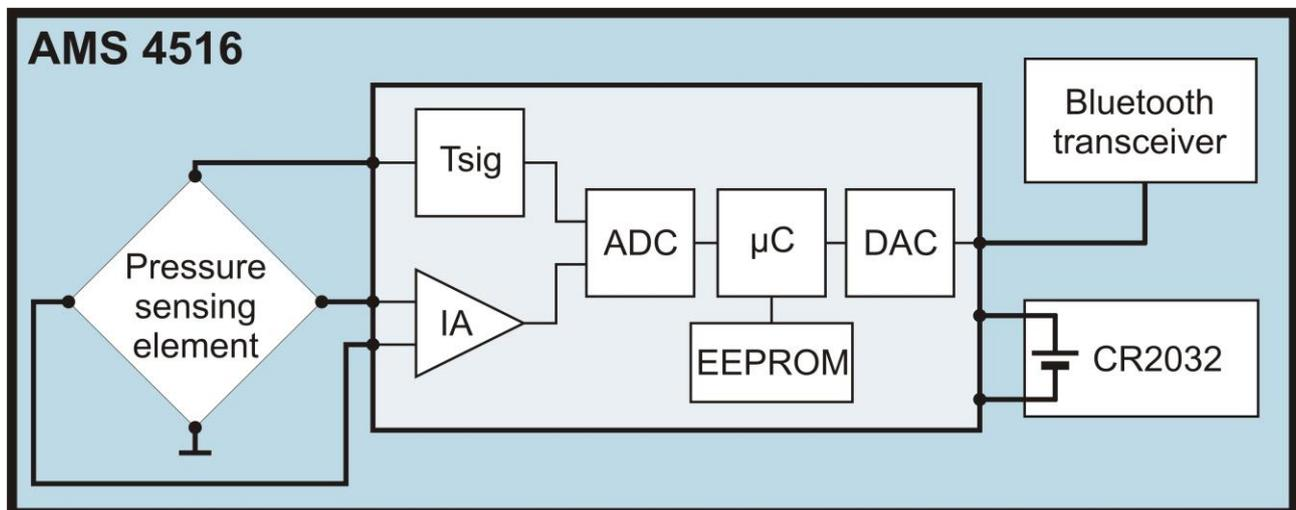
Figure 1: AMS 4516's block diagram
