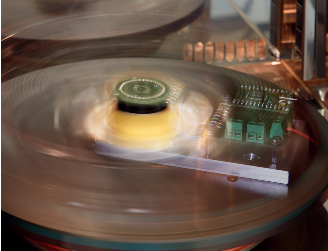
Characterization of a rotation rate sensor on the rotary table.
