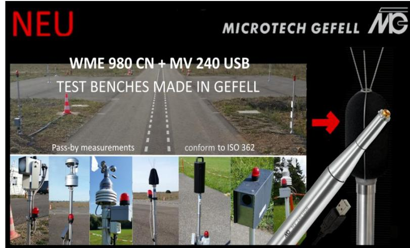
microphones with weather protection for temporary and permanent installations, especially for the automotive industry. The microphones are approved for official calibration/PTP certification and can be used for legally binding measurements. This means that the microphones are compatible with all common monitoring measurement systems and some are equipped with a remote calibration system.
