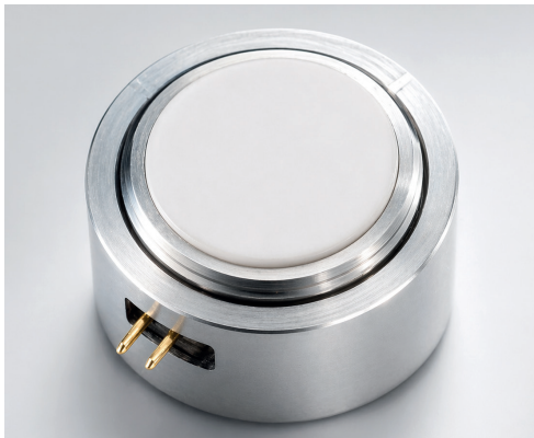
CMUT probe (assembled and packaged for high-temperature application).
