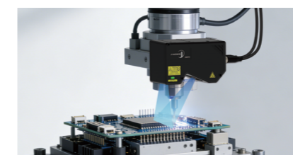
Dimension Inspection Gap measurement in robot assembly
