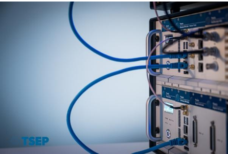
2: Trigger&Sync: TSEP has developed a product that coordinates the time synchronization between several TSEP THEMIS devices as well as between different plug-in cards within a single THEMIS device.
