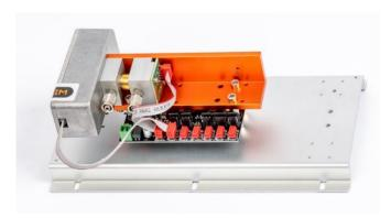
The entire signal processing takes place in an electronic evaluation unit (base board), which is located below the optical unit. Data is transmitted via an RS232 interface. CAN interface, MODBUS (option) and analogue output 0-10V (option) are also available.
