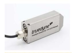
The sensor measures the density of liquids during the process itself, also in potentially explosive areas – no need to go to the laboratory. Thanks to a sub-millimeter measuring channel, the properties and quality of a liquid can be precisely monitored even in confined spaces.
