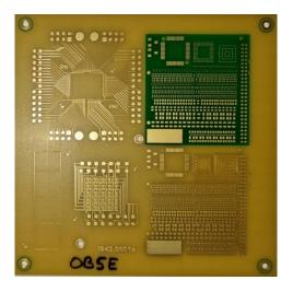
All PCBs were still functional even after 1000 thermal cycles, and no delamination could be observed on the PCB, on the solder mask or on the gold conductors.
